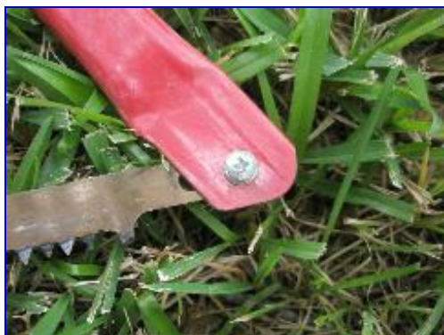
Rivet replaced with a nut & bolt
